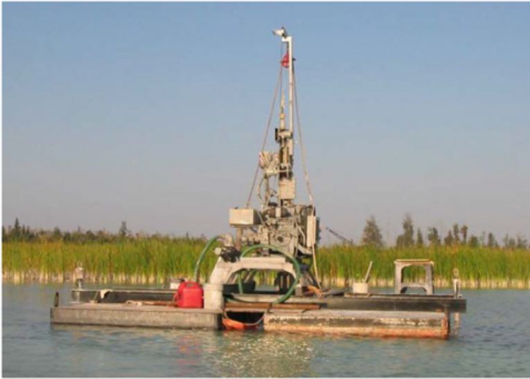
Figure 21-2. Drill and Barge Used for 2008 Fines Drilling Campaign.
