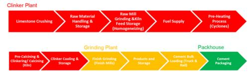
Figure 14-1. Cement Plant Process.
