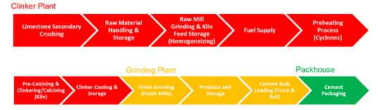
Figure 14-2. Cement Plant Process.
